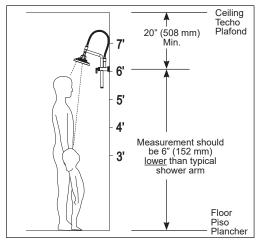
Select a height for the shower arm based on your personal needs. NOTE: Shower arm must be installed minimum 20" from the ceiling to prevent hose contact with the ceiling. The recommended distance from the floor is 6" lower than a typical arm to better access the adjustable arm.
